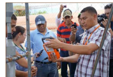
Measuring the percentage of methane in biogas during the RedBioLAC conference in Honduras. Photo taken in 2013 by Green Empowerment's Aaron Liss.
