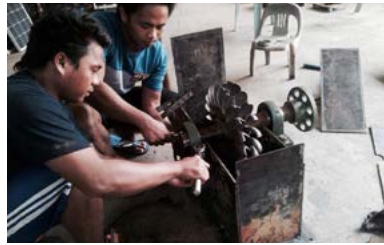
Trainees Denius and Aedon assemble a micro-hydro turbine at the CREATE center in Borneo. Photo by Green Empowerment's Gabe Wynn.
